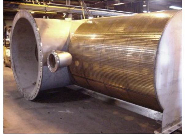
Tee Water Intake Screen
